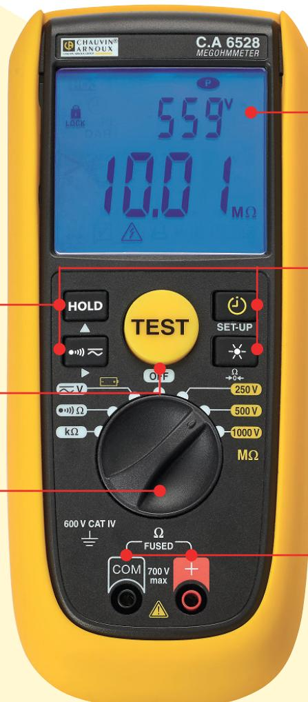
**HOLD:** automatic freezing of the display at the end of each measurement
