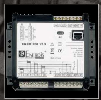
ENERIUM 110 and ENERIUM 210 non-display version available for DIN rail or plate mounting in cabinet
